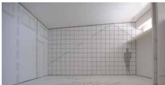
A less refined study model, at a larger scale, helps analyze the potential for natural daylighting in the classrooms – using a light-shelf on South windows – at the time of the SUMMER SOLSTICE. Similar documentation has been done at the time of the WINTER SOLSTICE. The goal is to limit electric lighting to overcast days or after sunset.
